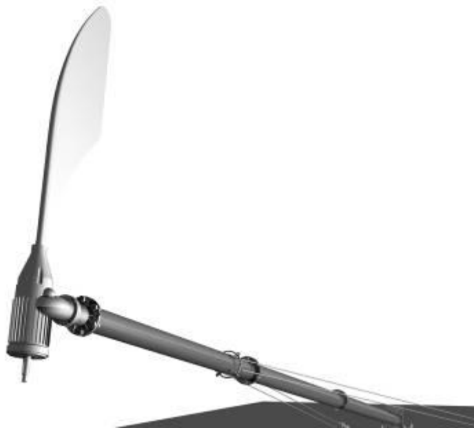
A) Peg graft the generator shaft to pole (or connect with flange), and screw fixed bolt
